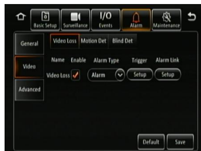
Video Loss Alarm Figure 103
